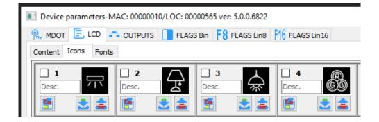
lcon files can be saved on your computer. Each icon comes with the option of opening the file, sending it to a device, or downloading it from the device. The icons can also be given descriptions.
