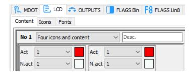
By default, an icon from the *N.act* row is shown. In order to display the icon for *Act* (active), a particular condition created in the *Device configurator* must be met. Once you have configured all the screens, it is necessary for you to click *Send* in the bottom right corner, in order to save the parameters in the device memory.
