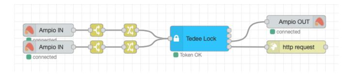
The block will expect the msg.payload string 'open' or 'close' at the input. This is why two Ampio IN blocks need to be attached – one for the 'open' flag, and the other for a 'close' flag. Then, attach the switch and change blocks. Switch verifies if msg.payload equals 1, while change sets the right 'open' or 'close' string.
