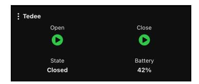
Updating the status and battery life can take a while – an update happens every 10 seconds. When you press the "open" or "close" buttons, the lock should perform those actions and update its status. When the open/close action is initiated with Ampio, the lock will keep updating every second for the next 10 seconds in order to report its status accurately. After that, it will start updating every 10 seconds again.
