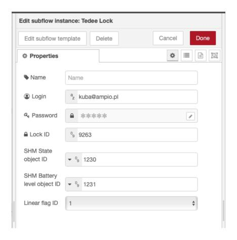
Enter your tedee account's login and password. Then open your lock in the tedee application and look for a gear icon at the bottom of the screen. Open the "Information" tab and copy the lock's ID into the block's parameters in Node-RED.
